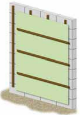
ANS fixing rails fixed to surfaces at 500mm centres
