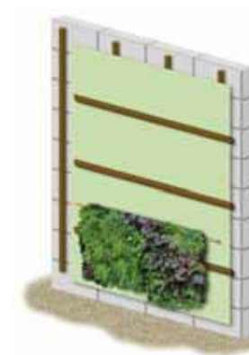
16mm diam. pipework with inline pressure compensated emitters at 125mm centres
